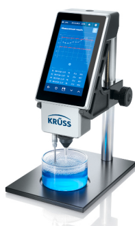
Bubble Pressure Tensiometer (BPT Mobile) - checks the cleaner or wetting agent content in a bath.
